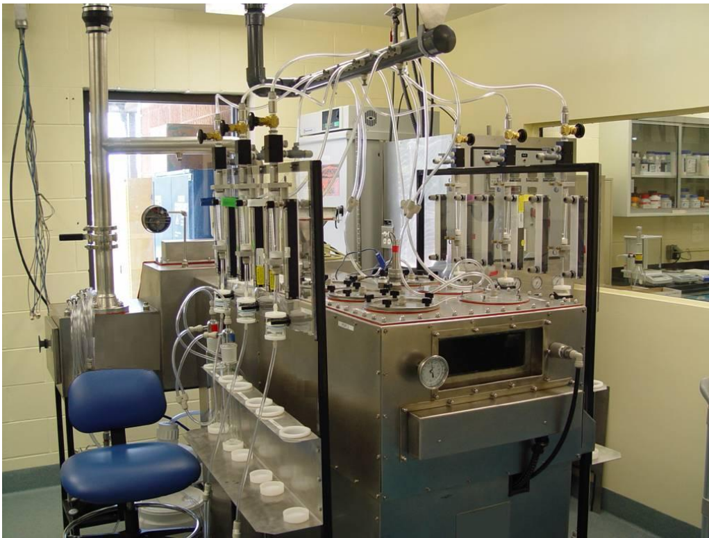
Figure 1. Top and Side View of BioAerosol Test System (BATS) Components.
