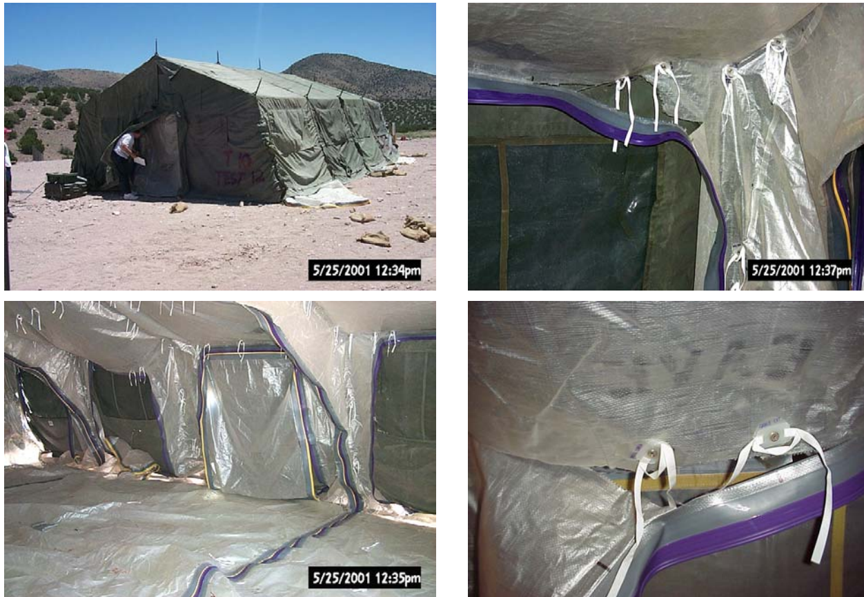
Figure 3. CPS liner failures. Clockwise from top, left: TEMPER tent with CPS liner lying outside the bottom of the tent 2 ; two photographs of tears in liners 2,1 ; failed zip seals 2 .
