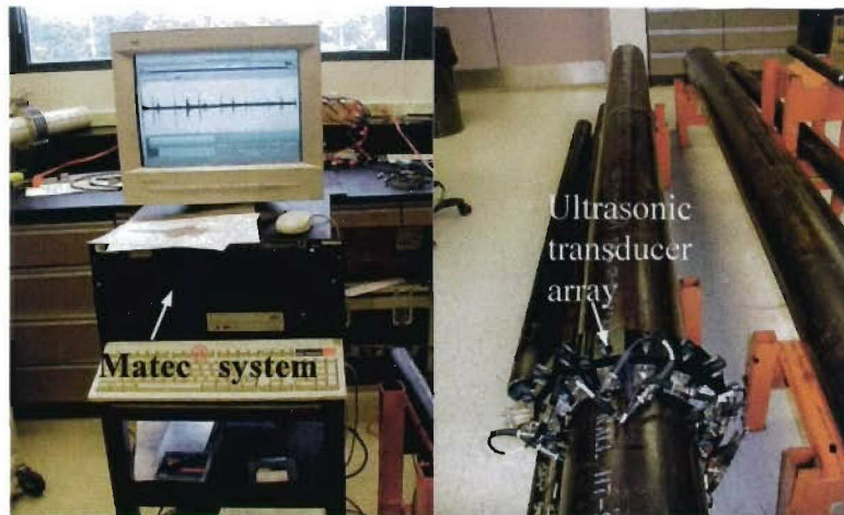
Figure 2-11. Experimental equipment, which includes the specially developed Matec ® ultrasonic A-scan 8-channel control system and a high frequency phased array on a 4" schedule 40 pipe for 200kHz~800kHz frequency tuning inspection.
