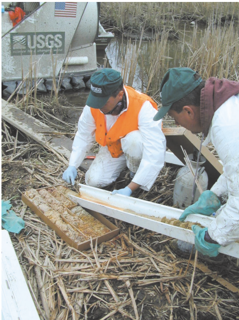
(C) Transferring the core into core boxes
