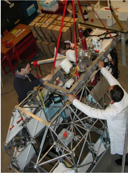
Figure 2-1 : An aeronomy stabilised gondola during integration (left) and ready for launch (right)
