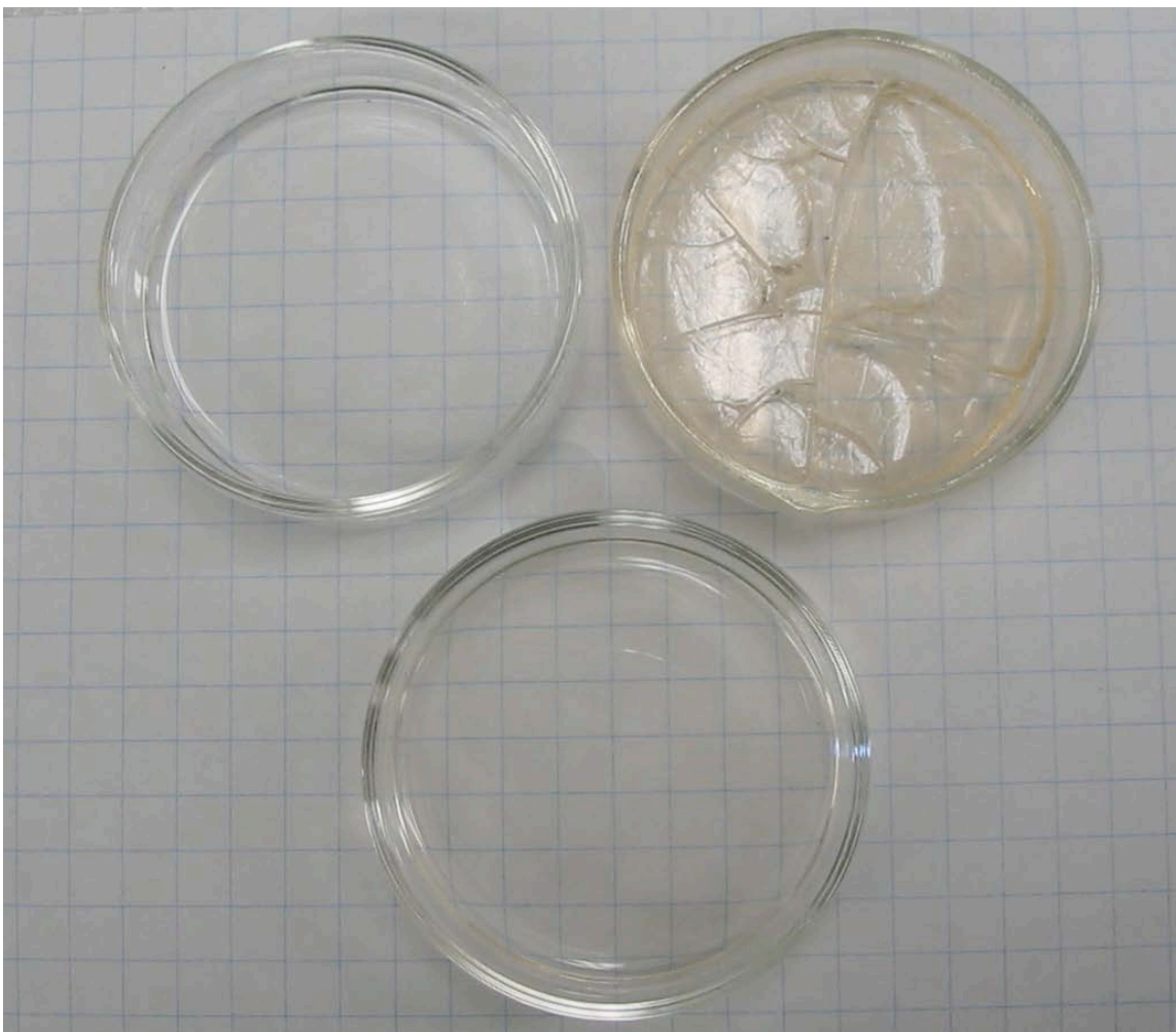
Figure 2.4 – Three dishes showing progressing reaction. First (top-left) is TMOS solution only. The second (lower) is liquid sol-gel with quantum dot added before condensation. Finally, the third (top-right) shows what happens when the reaction is too vigorous and gel quickly cracks.
