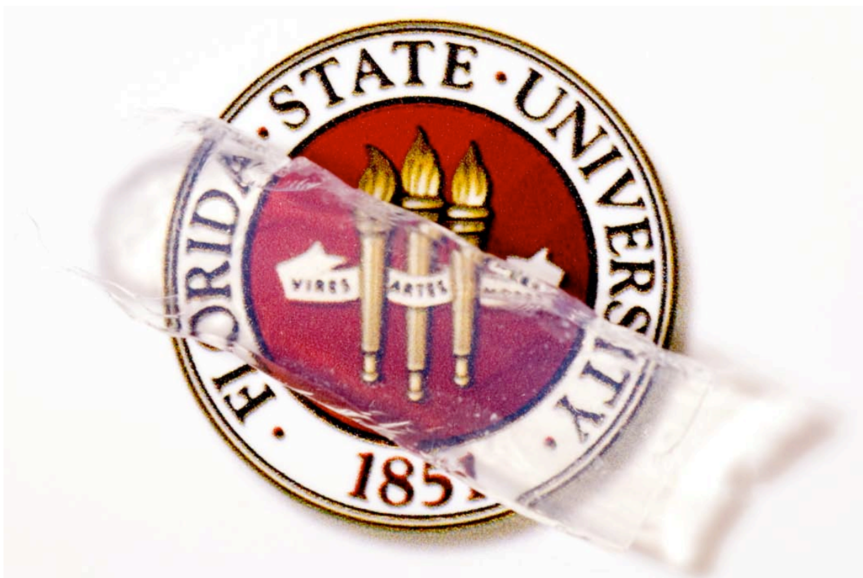
Figure 3.1 - Silica aerogel containing 2.5 nm CdSe/ZnS quantum dots.
