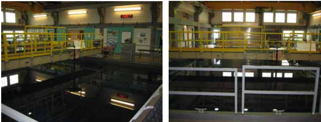
Figure 16. MBARI Test Tank Facility (Structure Above Water is Moveable Bridge).
