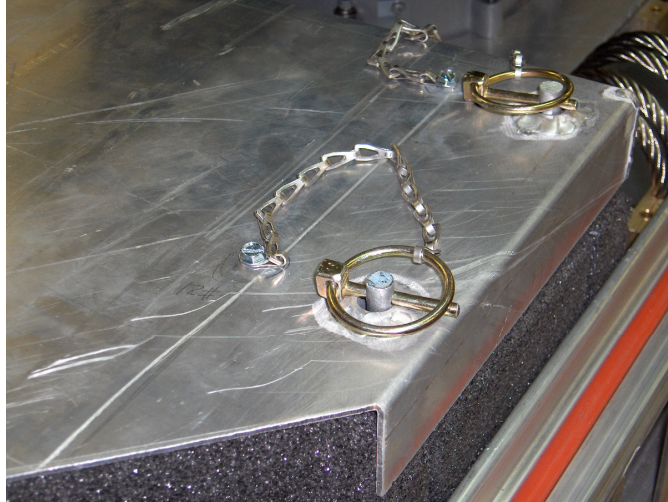
Figure 5. Three lynch pins hold the waveguide lid in place.
