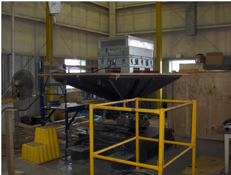
Figure 8. Resonance Dwell Test.
