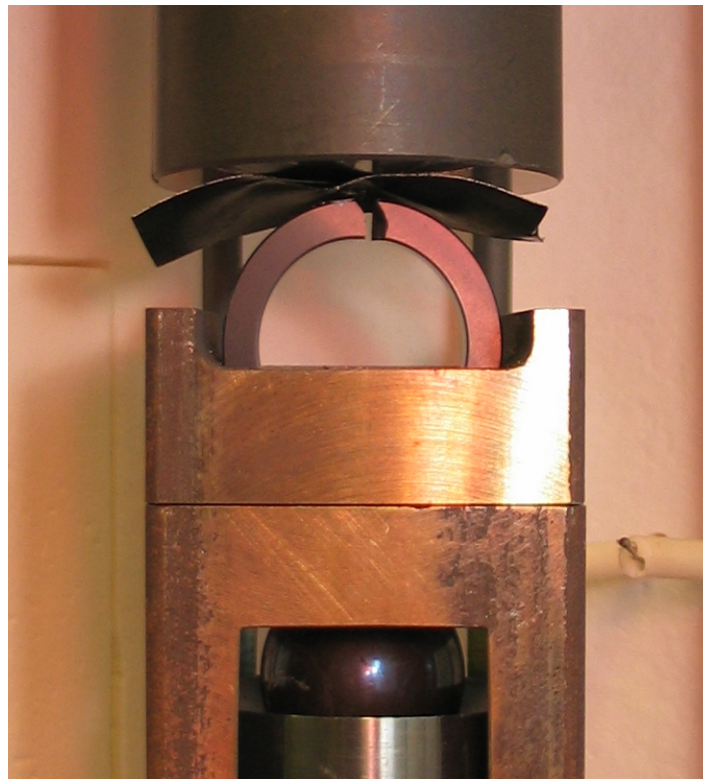
Figure 10. The 700 °C failed specimen.
