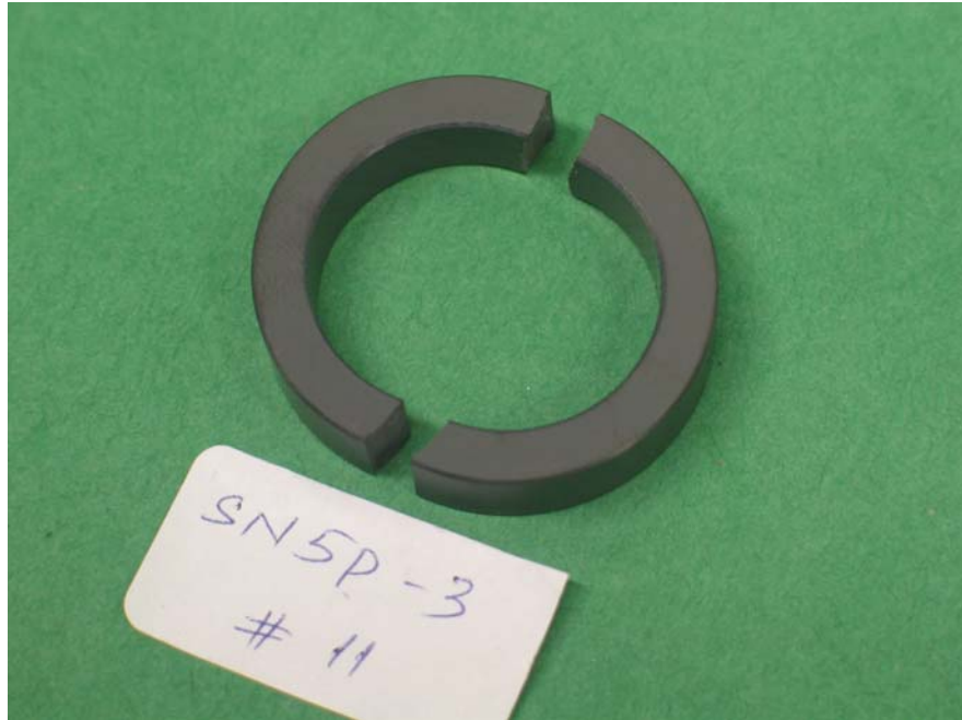
Figure 11. O-ring specimen fractured at 700 °C. The fracture pattern is indicative of a valid test.
