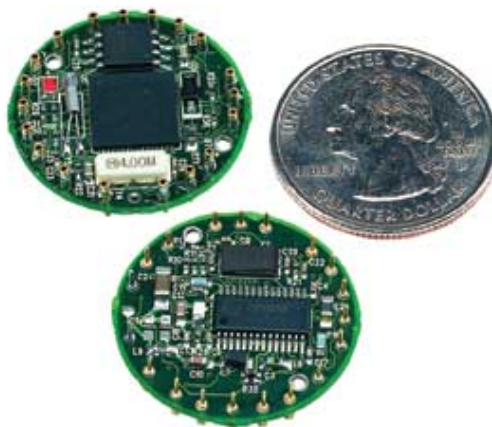
Figure 1. Crossbow MICA2DOT Quarter-Size Sensor (from Ref. [1])
