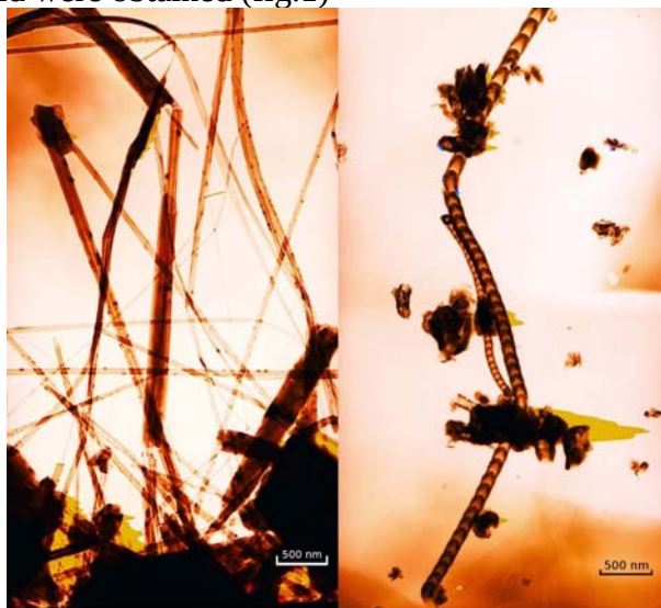
FIG. Electron-microscope images of BN-nanotubes. Bamboo structure (right) and variable diameter cylindrical (left)
