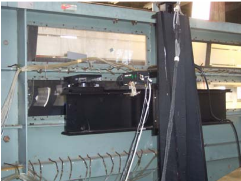
Figure 7. TSI camera mounted on the LDV mechanism.
