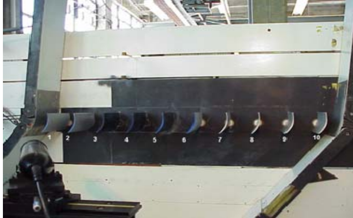
Figure 4. CD blades mounted in the LSCWT [From Ref 8].
