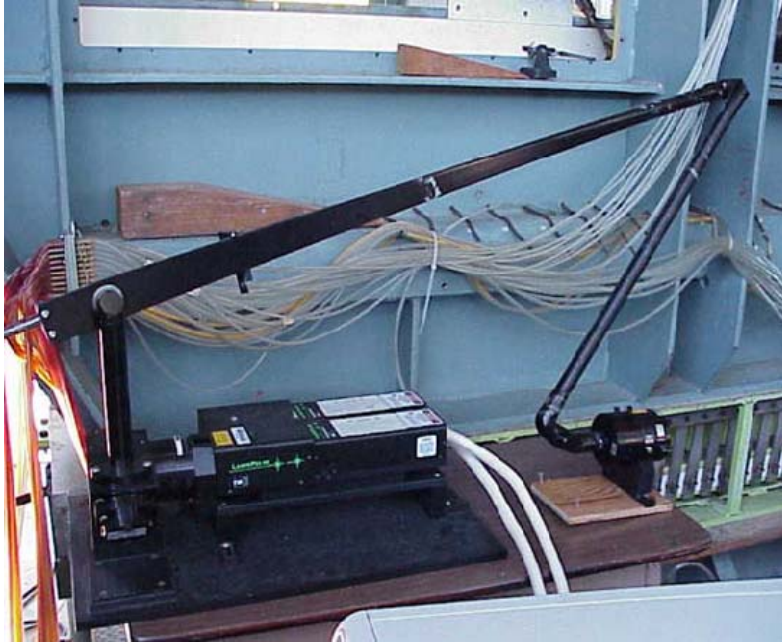
Figure 6. Dual Nd:Yag lasers and articulated arm with probe.
