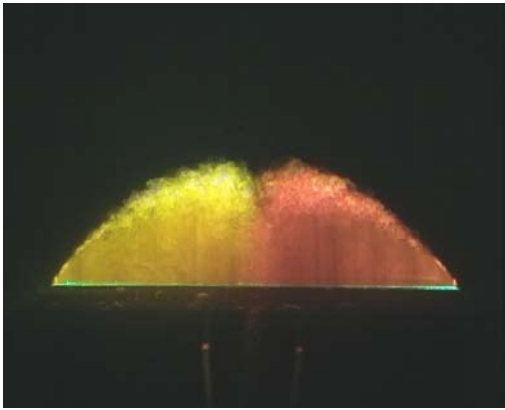
Figure 10: Time-averaged laser fluorescence flow visualization for stationary and rolling wings ( St=1.0 , \Delta\phi=1^\circ ).
