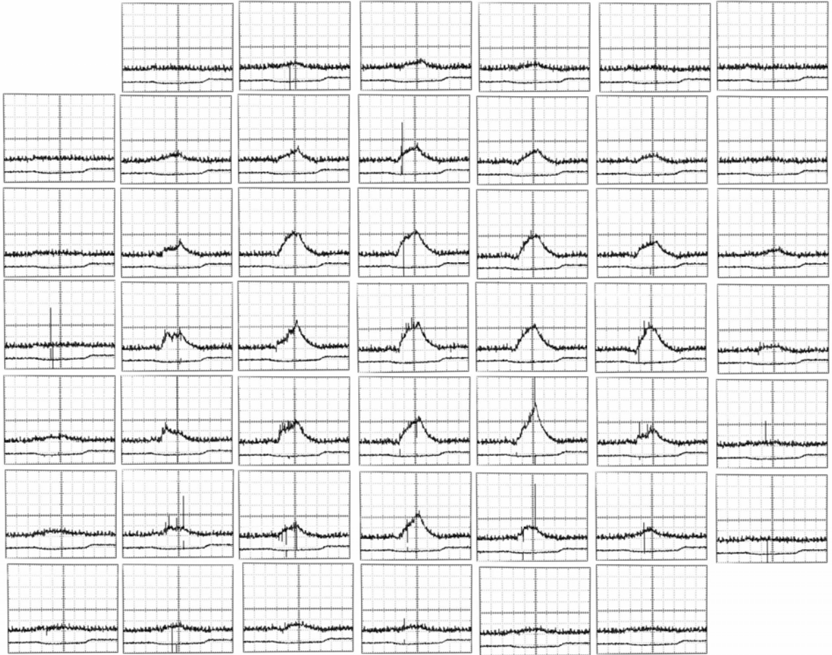
Fig.6.6.3. The measured waveforms T_{stag} in the control crosssection at air injection in the discharge area., p_{\Sigma} = 270 Torr. Upper waveforms - T_{stag} , lower waveforms -p_c
