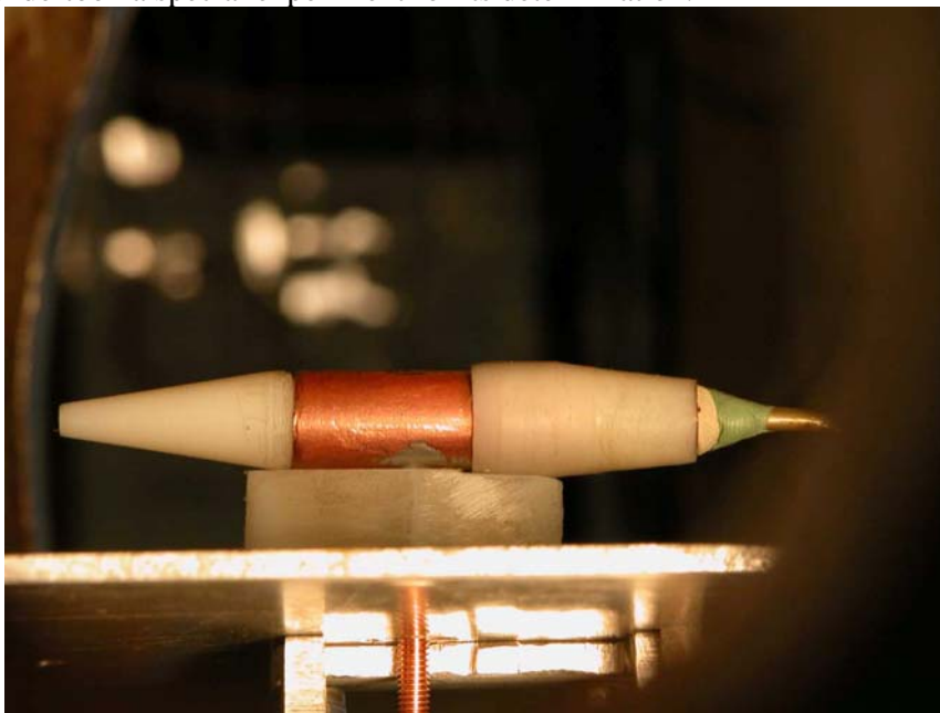
Fig.6.4.1. Photo of the mixer with attached Pitot tube
