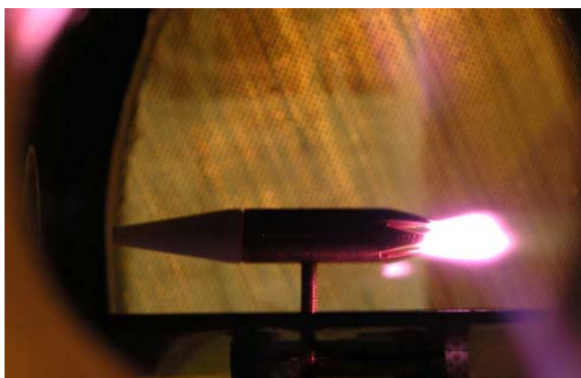
Fig.4.2.8 Discharge photo in vibrator base part with drawn in edges at exposure time \tau_{ex} = 1s
