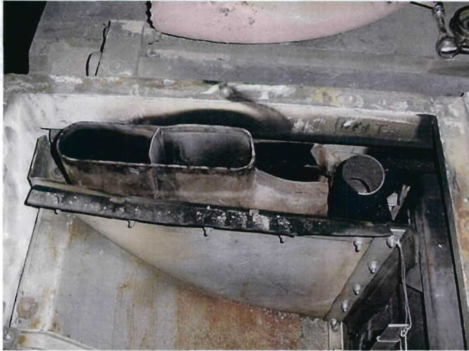
Figure 24 – Exhaust Gases Blow by the Exhaust Seal and Recirculate under Armor
