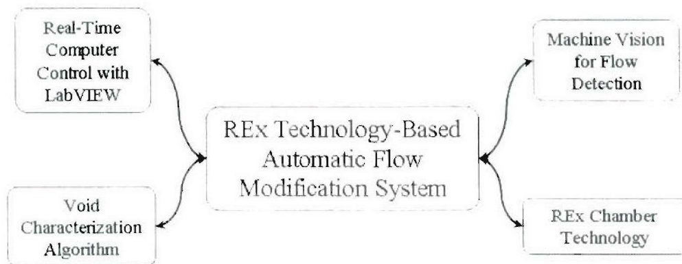
Figure 24 Main system components required for a flow modification system that utilizes an external vacuum chamber.
