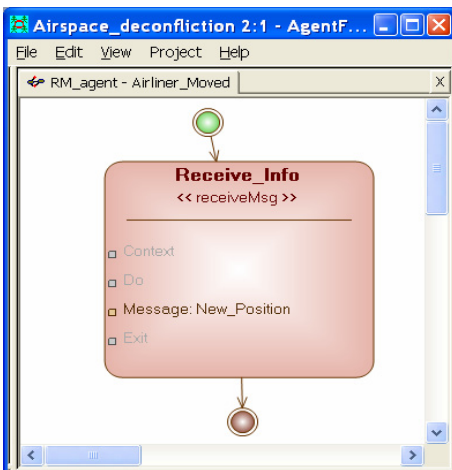
Fig.3.17. Specification of the Airliner_Moved service.
