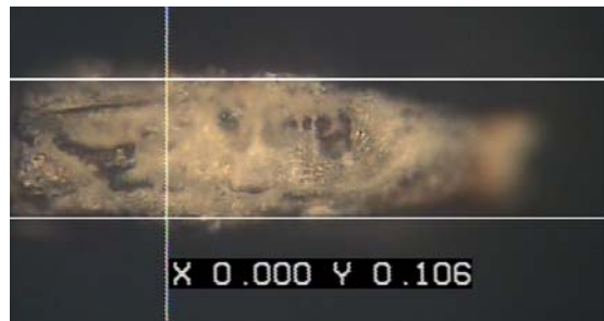
Figure 5.2(a) schematic of finger with vertical taper and (b) micrograph showing actual taper
