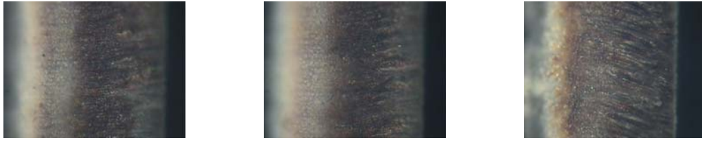
Figure 4.6 Exposed surfaces machined at rates of (a) 10mm/sec (b) 5mm/sec, (c) 2mm/sec, (d) 1mm/sec, (e) 0.5mm/sec, (f) 0.2mm/sec, (g) 0.1mm/sec, (h) 0.075mm/sec and (i) 0.05mm/sec
