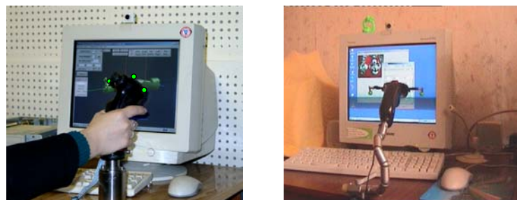
a). The 6D handle with force & torque sensor b). New HTS+ 6D handle ("Cober")
