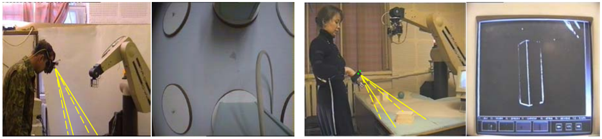
a).Camera mounted on helmet b).The image from camera on helmet c).Camera mounted on bracelet d).The image from camera on bracelet
