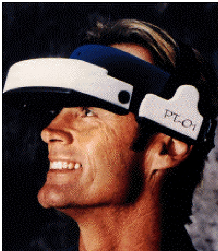
Figure 6- 5 - Portable EMAT System PT-01 Hardhat Mounted Computer Display
