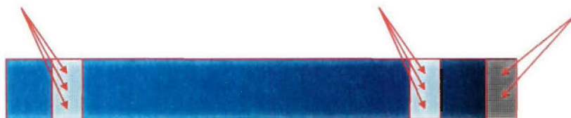
Figure 10. MgO in-plane texture for a meter long tape.
