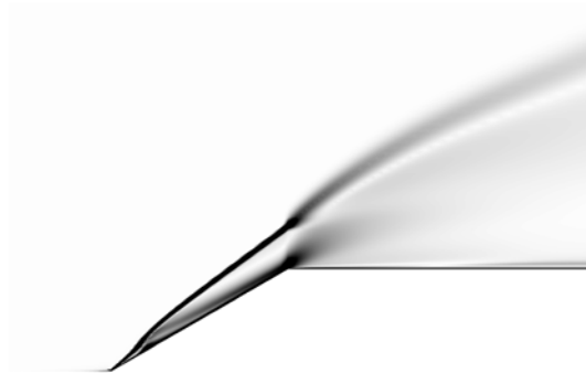
Fig. 3.17. The shadowgraph of the viscous flow in the magnetic field with electric current through the electrodes (configuration 4)
