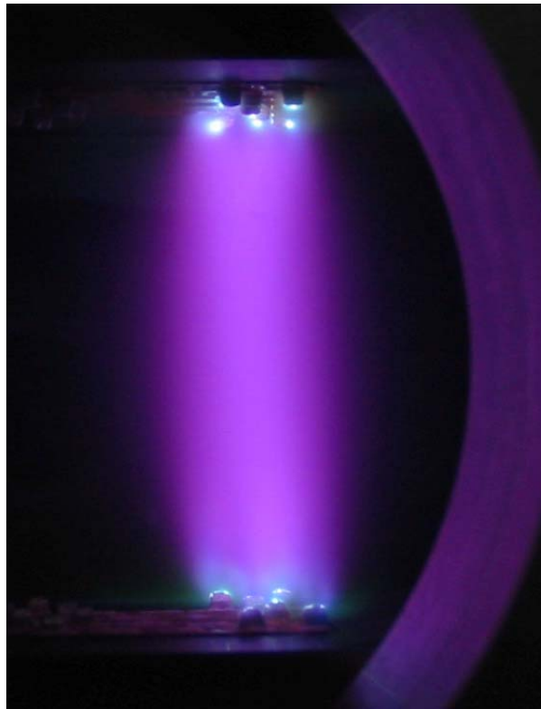
Fig.1.1.8. Photograph of luminosity in one-pulse high-voltage discharge
