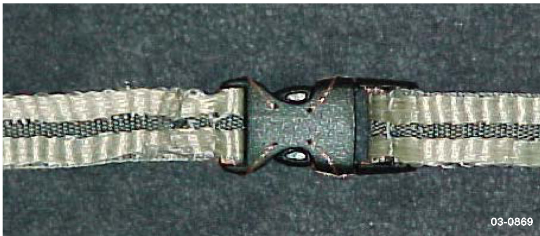
Figure 5. Bottom view of buckle concept for power transmission using loosely woven Aracon bus
