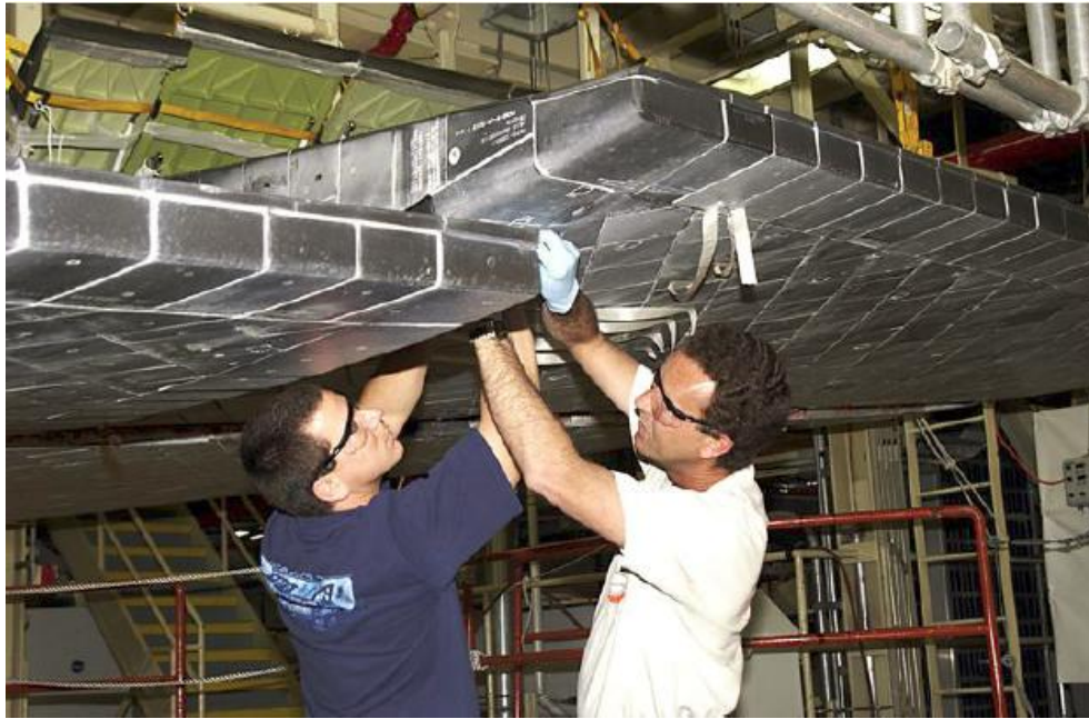
Figure 1 Thermal Protection Repair Activity around Orbiter Elevon Aero surfaces McCleskey, C. M. (2005)
