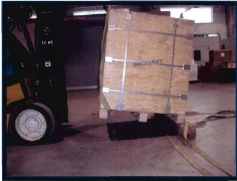
Photo 7. Edgewise Drop Test on the Test Unit.
