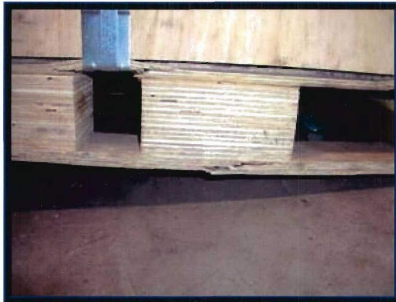
Photo 8. Minor Damage Sustained During Drop Test.
