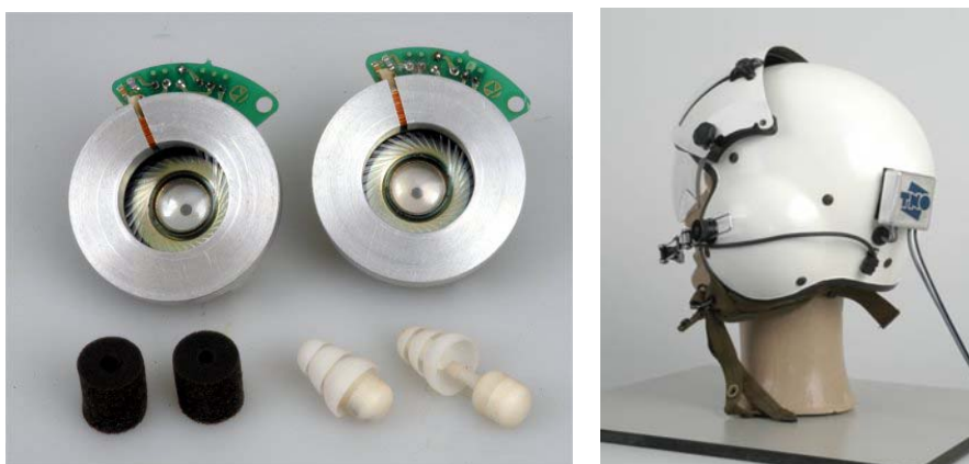
Figure 10. Earcoils and wireless earplugs (left) and helmet with w-CEP electronics (right) used in wireless CEP field evaluations. The earcoils, with integrated conventional earphones for backup purposes, are built into the earcups of an existing helmet or headset. The helmet with w-CEP electronics is connected to an intercom system in the usual way.
