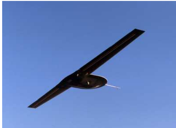
Figure 1.1: The DarkStar is a unmanned combat aerial vehicle intended to operate as a stealth attack platform.
