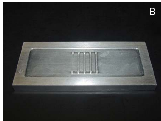
Figure 4. Aluminum PDMS molds containing (A) five lanes that are 800 \mu\text{m} wide, 250 \mu\text{m} high, and 15 mm long; and (B) 800 \mu\text{m} wide, 15 mm long, and varying in height from 25 \mu\text{m} (far left) to 250 \mu\text{m} (far right).
