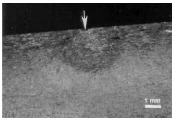
Figure 9 – Fatigue fracture surface of typical machined + 100hr salt fog exposure sample. Arrow indicates fatigue origin at the site of corrosion pit.
