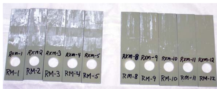
a. Non-wiped and wiped subgroups after one test cycle
