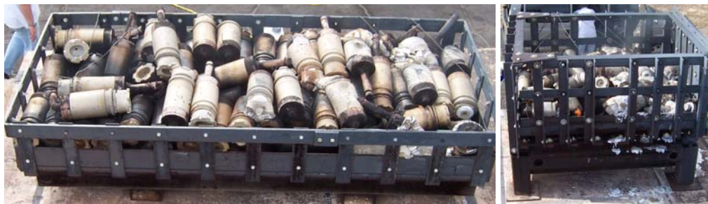
Figure 18: Baskets R1 and B1 respectively show no visible signs of deformation after initial testing.
