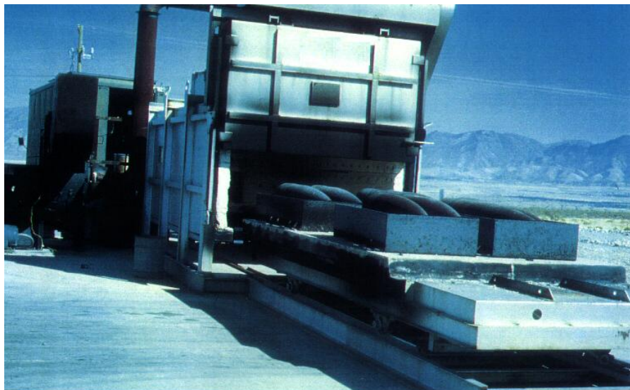
Figure 1: The US Army simple flashing furnace with a rolling hearth (processing 750 lb. bomb shells)
