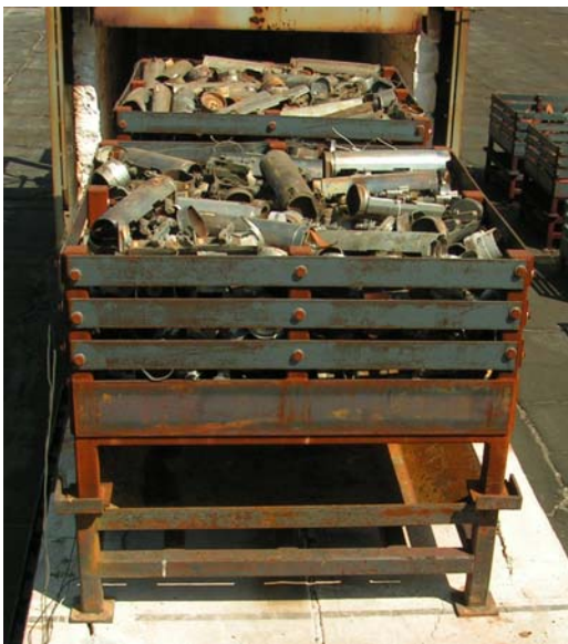
Figure 7: Two baskets each filled to maximum volumetric capacity of range scrap each are flashed in the same heat cycle.
