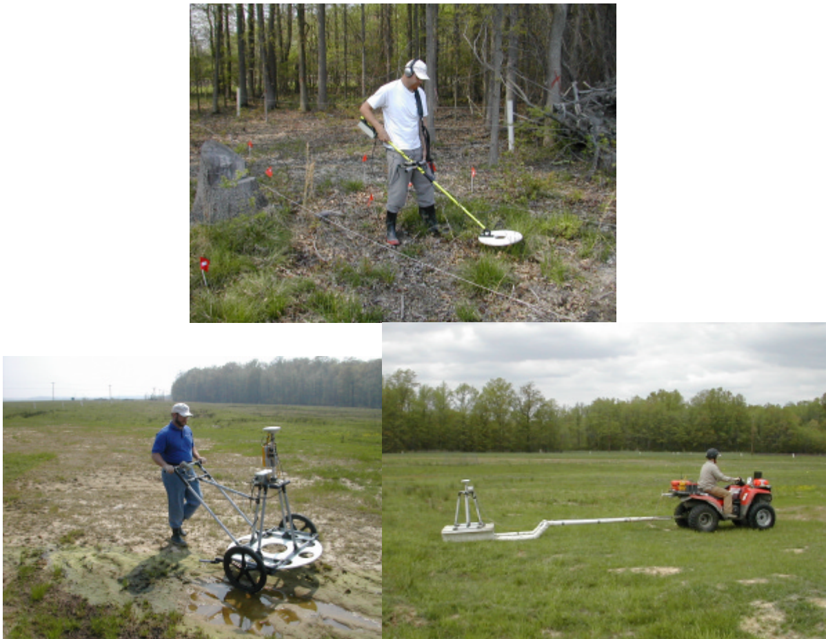
Figure 2. The GEM-3 can be either handheld, or cart/sled-mounted and pushed or towed
