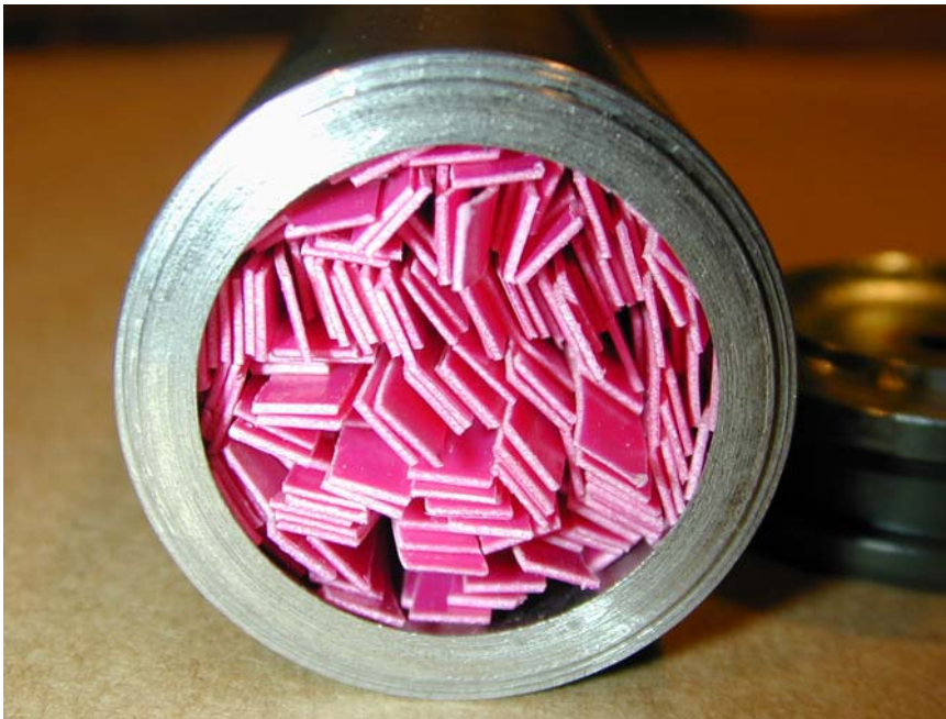
Figure 11: TGD-044 co-layered ribbon grains in 25 mm case, breech end.
