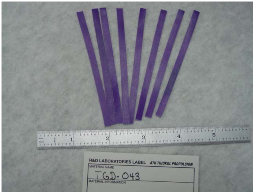
Figure 7: TGD-043 co-layered ribbon grains.
