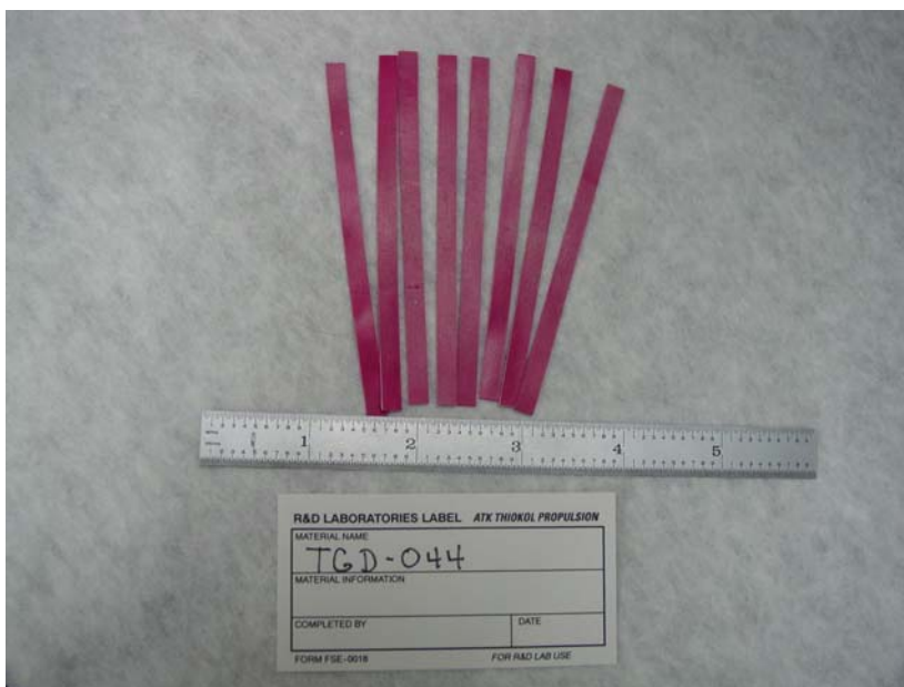
Figure 9: TGD-044 co-layered ribbon grains.
