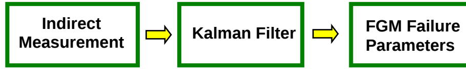
Fig. 4. Schematic of inverse analysis to determine failure
