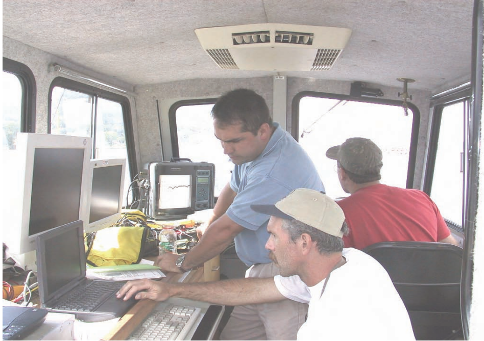
Figure 7. Survey boat on-board computers, which provide boat location and monitor all data collection activities for multi-beam and ADCP instrumentation
