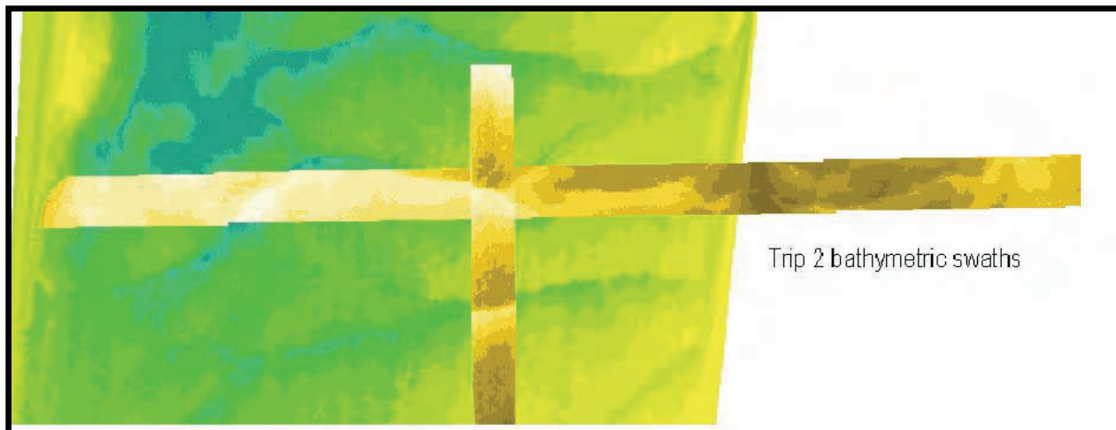
Figure 11. Contoured plot of cross-wise and longitudinal swaths of bathymetric data, Pool 8
