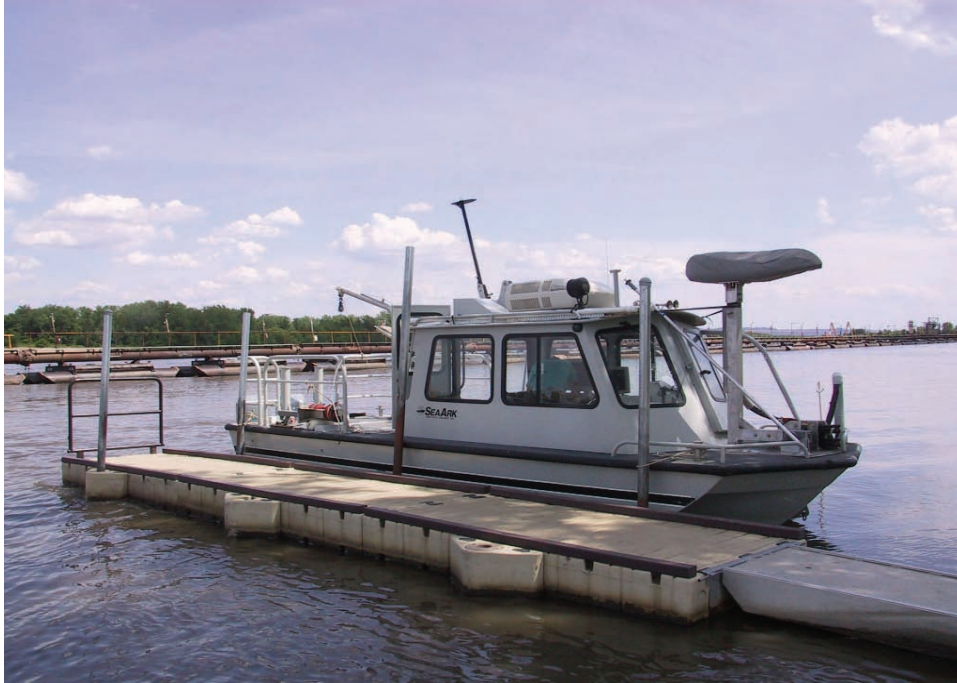
Figure 6. Survey boat for acquiring hydrographic, sediment, and bathymetric data
