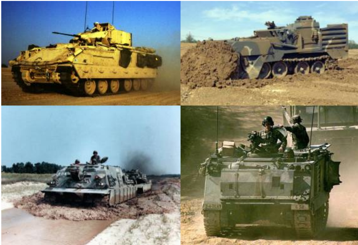
Figure 2. Examples of tracked vehicles: Top left, a Bradley fighting vehicle; top right, an M9 combat earthmover; bottom left, an M88 Hercules recovery vehicle; bottom right, an M113 armored personnel carrier (APC).
