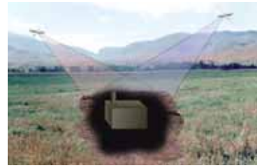
Figure 4: Realistic scene with an elevated (aerostat) airborne receiver, and a subsurface radiator to facilitate precision engagement. Figure 5: UAV based bistatic GPR for subsurface facility detection.
