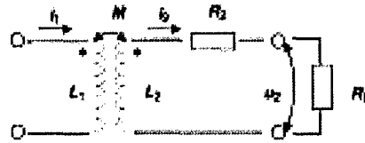
FIG. 3. Continuous energy transfer to inductor loop 2
