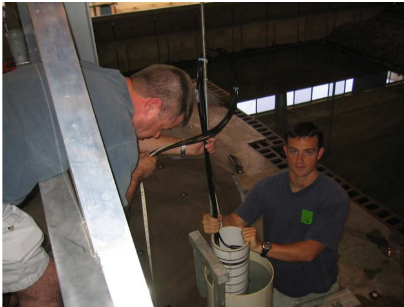
Figure 13, Pressure sensor calibration
