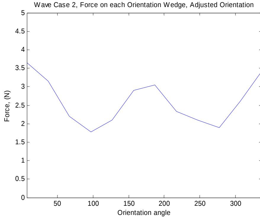
Figure 59, Force on each wedge orientation, case 2
