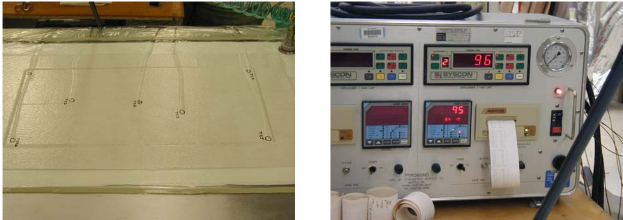
Figure 4.3-1 Vacuum bag assembly and temperature controller
