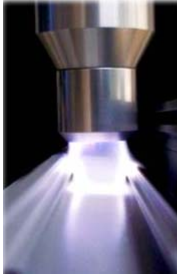
Figure 4.1-4 Plasma head used for pretreatment of metal alloys
