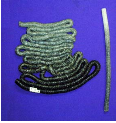
Figure 4. Graded Composites manufactured using the TSE process
