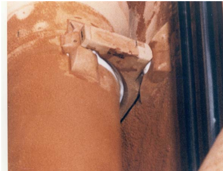
Figure 2. Ice frost on a LO 2 feed line bracket of the external tank.
