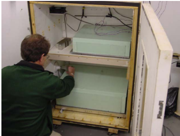
b. Insulated cover to isolate the samples inside the cold box for maximum temperature stability.
