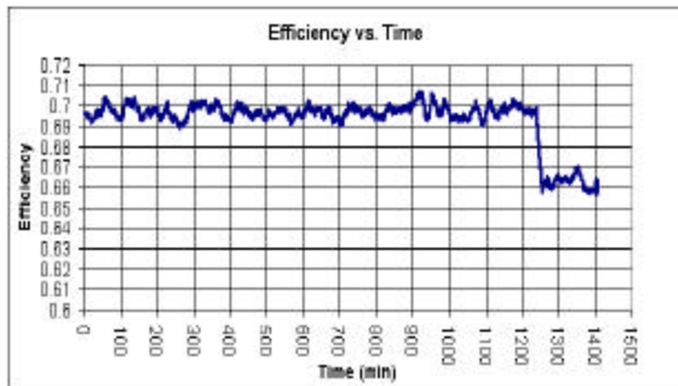
Figure 10 - Efficiency vs. Time During BJT Failure
