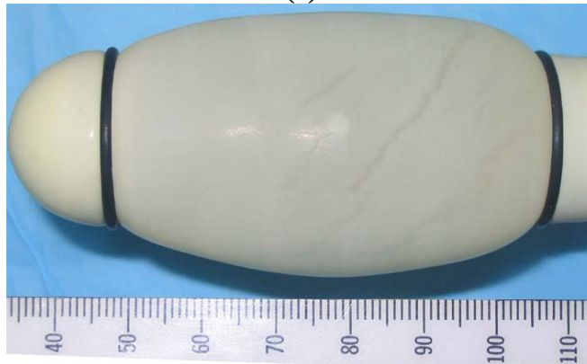
Figure 21: A photograph showing the transrectal probe utilizing prototype array #2, after assembling the soldered array and the appropriate brass tubes into the MRI compatible housing.
