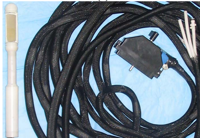
Figure 22: A photograph showing (a) the inflated water bolus of the transrectal probe and (b) the probe with its 10.5 m electrical cables and air and water circulation hoses.
