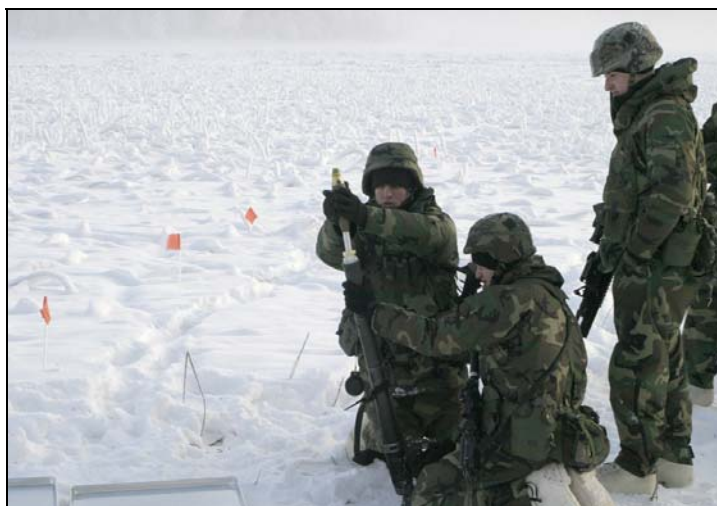
Figure 4. M19 mortar and M888 cartridge with a single M204 propellant charge.
