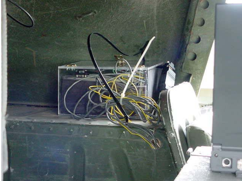
Figure 7. Data Acquisition System Mounted on Left Rear Wheel Well
