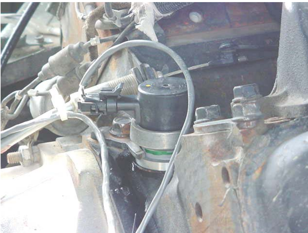
Figure 3. Installed Tachometer Drive
