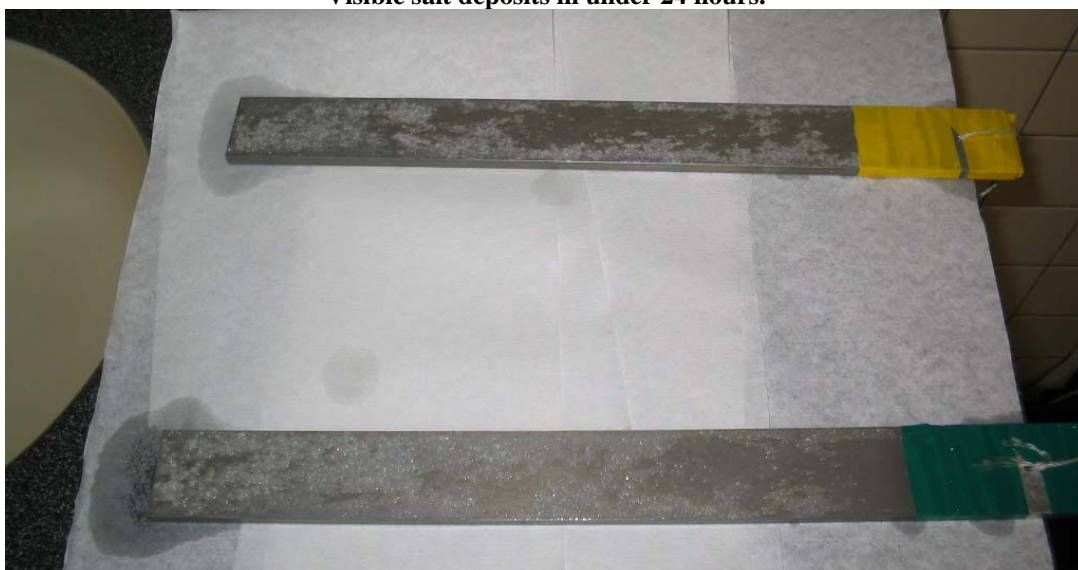
Figure 184. Fronts of green and yellow beams after corrosion. White markings are salt deposits.
