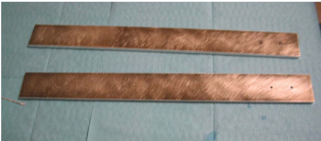
Figure 197. Red notchless beam on top, white/red notched on bottom. Front surfaces before corrosion
