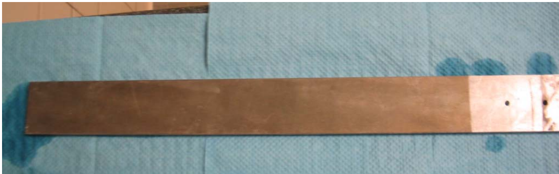
Figure 220. Front of white notchless beam after corrosion and cleaning. Note that mostly general corrosion is present.
