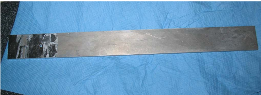
Figure 208. Back of blue/green notched beam after cleaning.
