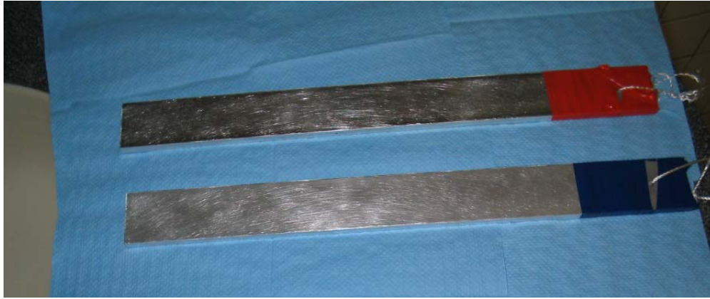
Figure 190. Blue notchless and red middle notched beam before 48 hour corrosion
