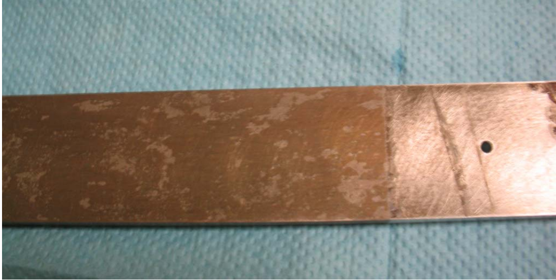
Figure 216. Front of yellow/blue notched beam (clamp end) after corrosion and cleaning
