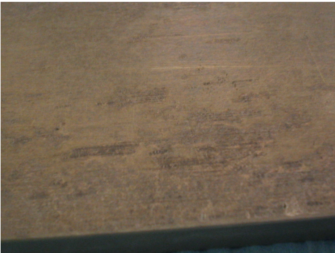
Figure 189. Zoom in on back of yellow cleaned beam. Overall corrosion and some apparent pitting despite the lack of salt deposits.
