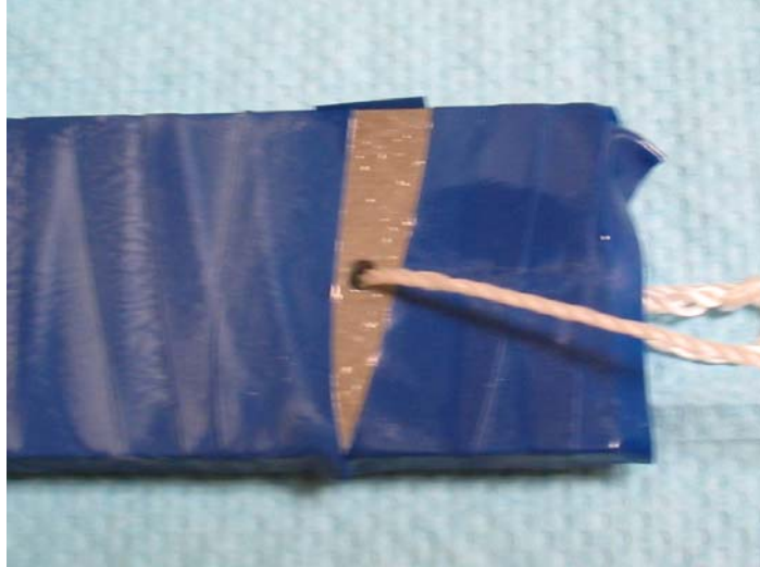
Figure 192. Salt deposits present on non-immersed portion of exposed beam
