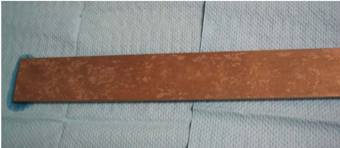
Figure 217. Front of yellow/blue notched beam after corrosion and cleaning
