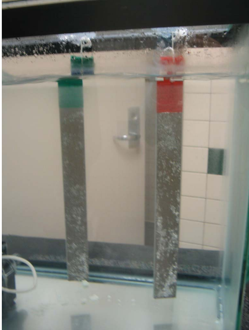
Figure 202. Beams in the tank, salt deposits evident on this side
