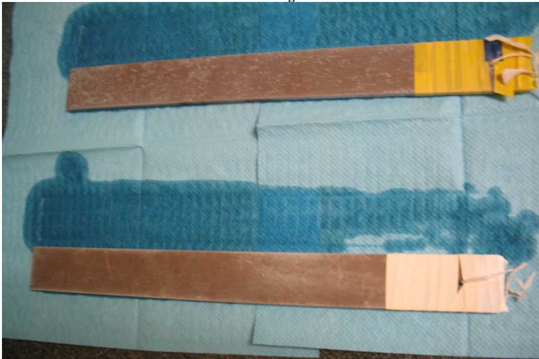
Figure 215. Back of yellow/blue middle beam, front of white notchless beam after corrosion, before cleaning
