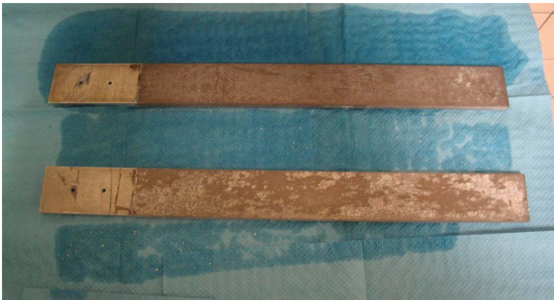
Figure 205. Back of beams after corrosion, before cleaning. Blue/green middle notched beam is on top, white/red notchless beam is on bottom.
