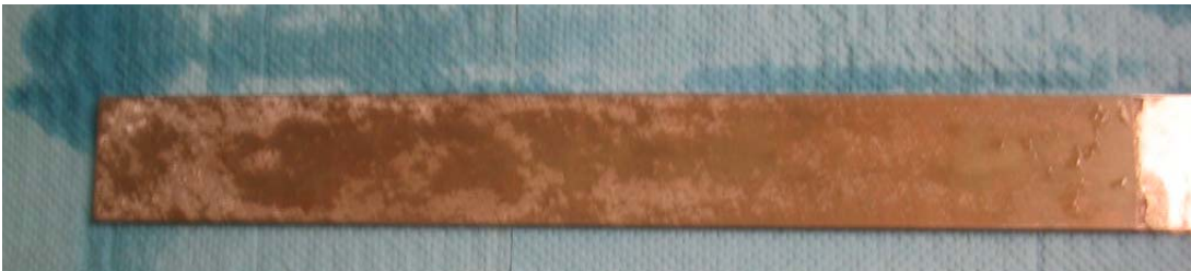
Figure 221. Back of white notchless beam after corrosion and cleaning. Lighter gray areas indicate former presence of alt deposits.
