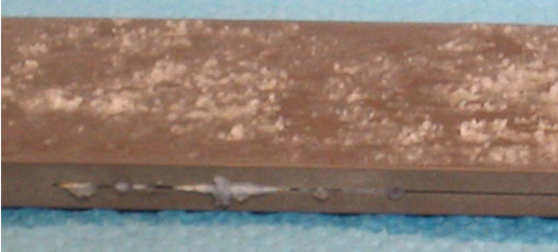
Figure 206. Zoom in on corrosion product in notch.
