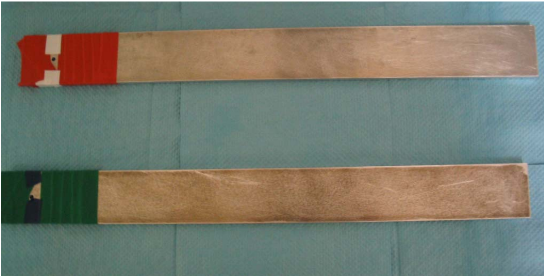
Figure 201. Back of white/red notchless and blue/green middle notched beams before corrosion.
