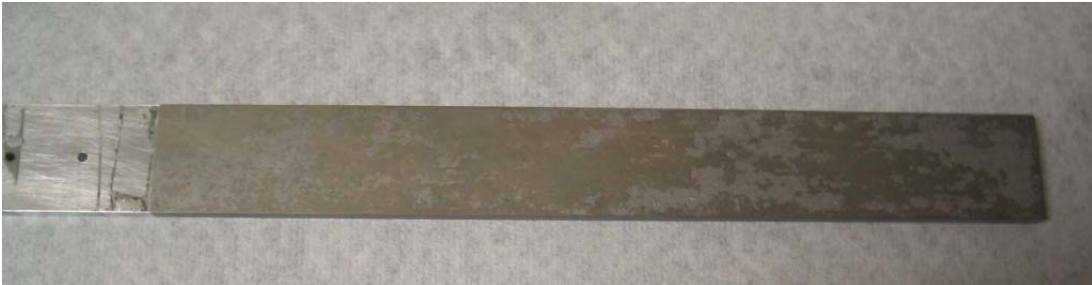
Figure 210. Back of white/red notchless beam after cleaning.
