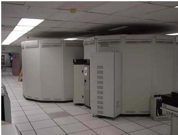
Figure 4. Tertiary storage tape silos at USC.
