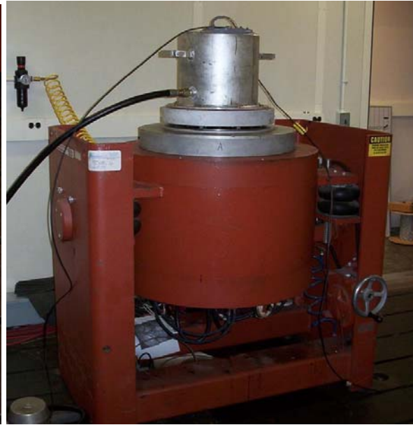
Figure 27. Vacuum Pump and Pressure Gauge Figure 28. Experimental Set-Up on 18k lbf Shaker
