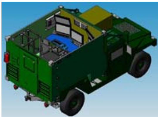
Figure 2: OCU located in back of HMMWV with multiple screens and racks of computers to run C2 software.
